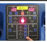
STEP 5 With the engine running, and a fluid pressure of 3 to 50psi, press the COOLER LINE button. This will allow transmission fluid from the transmission pump to pass thru the equipment and back to the transmission. The NEW fluid level will default to 12.0 Qts and the Waste fluid level will default to Zero Qts...
