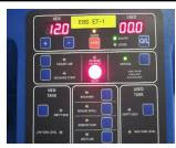
STEP 4 Start the vehicle. Fluid pressure should increase on the pressure gauge and the READY light will turn on. If the pressure does not increase, IMMEDIATELY turn off the vehicle and reverse the hose connections (see STEP 2) and re-try. If the vehicle is cold and a thermostat is involved it may be necessary to warm up the vehicle.
