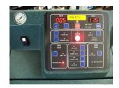
STEP 3 Connect the unit's power cord to a 110vac outlet. Use a heavy duty extension cord if necessary. Turn the power switch on the lid on. The control pad screen should light up and then show old and new fluid amounts in each tank. Fill NEW Tank or empty USED Tank as required.
