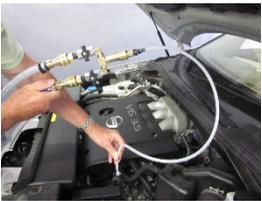
**STEP 10** Remove dipstick hose from vehicle. Replace dip stick and start vehicle. Check Transmission fluid levels and correct using the VAC or FILL Switch as appropriate. Transmission service is complete.
