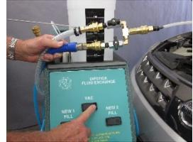
**STEP 4** Shut off engine and insert the largest Diameter dipstick hose into the dip stick tube as far as possible and attach the Vacuum Service Hose to the dipstick hose. Use the hanger to locate the SCH conveniently under the hood.
