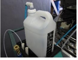
**STEP 8 - Trans Service -** Start engine. Run engine for approx. 30 - 40 seconds while going thru the gears to circulate NEW Fluid. Turn engine OFF. Perform STEP's #5 and #7 again then go to STEP #10
