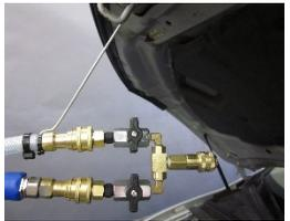
**STEP 9 – Oil Service -** After STEP #7, remove equipment dip stick hose. Check Oil levels and correct using the VAC or FILL Switch. Replace old Oil Filter. Oil Service is complete.
