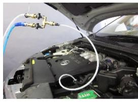
**STEP 5** Turn all switches on the control panel OFF. Connect the power cord to a 110vac outlet. **ENGINE IS OFF.** Turn the VAC switch ON and vacuum as much fluid from the reservoir as possible. Turn the VAC switch OFF.
