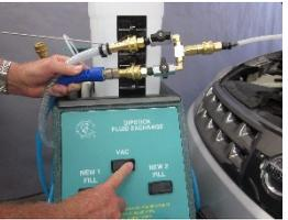
**WARNING:** Once a particular type of fluid, for instance transmission fluid (ATF) has been used in a TANK, do not use another type of fluid (like OIL) in the same TANK for another service. Damage to the equipment and the vehicle is probable.
