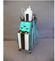
**STEP 6** Examine the condition and amount of old fluid removed. If large particles or black fluid has been removed determine if the vehicle system is damaged and correct or repair before proceeding.
