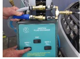
**STEP 2** Start with an empty waste tank as checking the amounts of fluid removed from the vehicle is necessary for proper service. Waste tank is marked in qt levels. Attach the Cap hose assembly in the top shelf to the Waste Tank.
