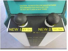
**STEP 7** NEW FILL 1 or 2 switch ON. Monitoring NEW TANK levels replace the fluid amount removed in STEP 5 plus a ½ quart to compensate for fluid in hoses. Turn NEW TANK FILL switch OFF. **OIL Service - Go to STEP 9**
