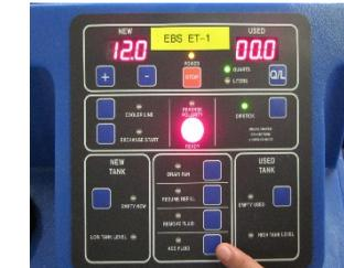
**STEP 5** With the engine running, and a fluid pressure of 3 to 50psi, press the COOLER LINE button. This will allow transmission fluid from the transmission pump to pass thru the equipment and back to the transmission. The NEW fluid level will default to 12.0 Qts and the Waste fluid level will default to Zero Qts..
