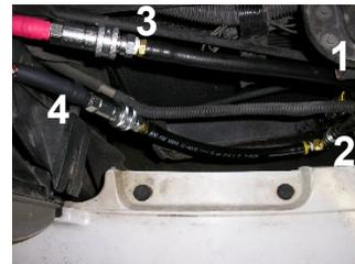
**STEP 7** Press the EXCHANGE START button. The equipment will exchange fluid from the transmission in 2 tenths of a quart increments until the total selected in STEP 6 is exchanged. As the fluid is being exchanged the NEW fluid level will be decreasing as the WASTE level is increasing.
