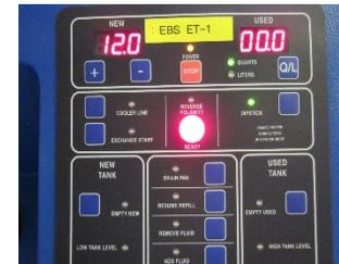
**STEP 4** Start the vehicle. Fluid pressure should increase on the pressure gauge and the READY light will turn on. If the pressure does not increase, IMMEDIATELY turn off the vehicle and reverse the hose connections (see STEP 2) and re-try. If the vehicle is cold and a thermostat is involved it may be necessary to warm up the vehicle.
