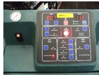
**STEP 9** Check the transmission fluid level. Add or remove fluid as necessary by selecting ADD FLUID or REMOVE FLUID button on the control panel. Select the desired amount using the "+" or "-" buttons. Press the ADD FLUID or REMOVE FLUID button again to start that process.
