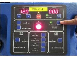
**STEP 12** Repeat STEP 6 thru STEP 11. Upon completion start the vehicle, check fluid levels, and adjust as necessary using the ADD or remove fluid using the DIPSTICK service tube. Remove service tubes and hoses.
