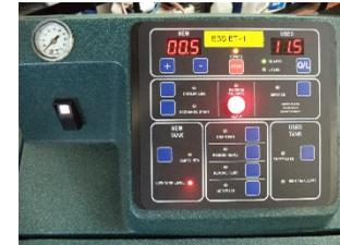
**STEP 3** Connect the unit's power cord to a 110vac outlet. Use a heavy duty extension cord if necessary. Turn the power switch on the lid on. The control pad screen should light up and then show old and new fluid amounts in each tank. Fill NEW Tank or empty USED Tank as required.
